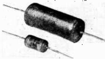
Hunt's metallised paper capacitors; showing one of 0.1 \mu\text{F} and one of 0.5 \mu\text{F} capacity. As the larger is comparable in dimensions to a standard pattern paper tubular of 0.1 \mu\text{F} it serves as a basis for comparing the size of the smaller 150-volt type. The larger is for 350 volts DC working.
